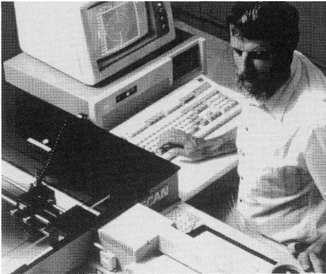
Figure 3. Two-Dimensional (2-D) Radiochromic Film and Plate Scanning Dosimetry System Exposed radiochromic film can be seen in the lower left-hand corner of this photograph. (Courtesy of AECL Research, Ref. 30).
